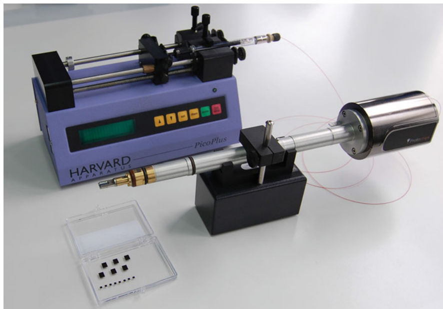
Fig. 9.3 Liquid flow specimen TEM/STEM holder system (“Poseidon” Protochips Inc., NC., USA). Microchips in a box are shown at the lower left corner . A microfluidic syringe pump (Harvard Apparatus, MA, USA) is connected to the holder via plastic tubing (Upchurch Scientific PEEK Tubing). With permission from (Schuh and de Jonge 2014)
