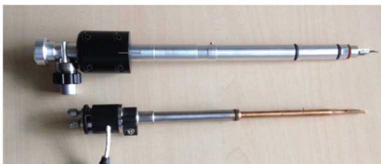
Fig. 6.3 A comparison of the shapes of a JEOL and an FEI flowing gas holder
