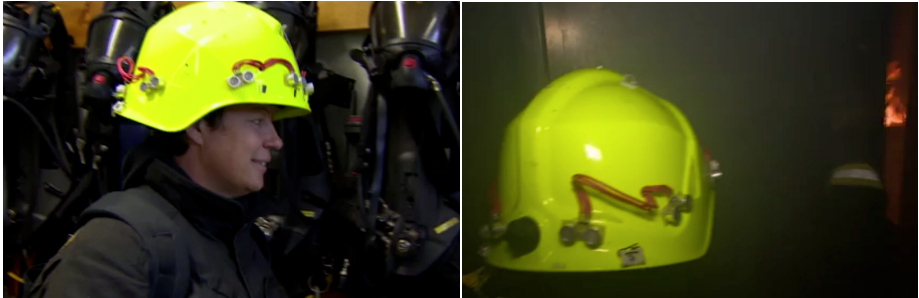
Fig. 1. Ist generation Tactile Helmet design undergoing field testing. In right-hand picture the fire-fighter is in a confined smoke-filled space in the South Yorkshire Fire and Rescue training facility.
