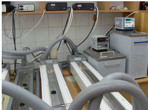
Fig. 5.1 A set for automatic registration of snail thermal preferences. Snails move in a chamber with an oblong thermal gradient (temperature range: +8 to +38 °C). The position is recorded by the infrared sensors connected to thermocouples. The data are transferred to a computer and stored by GRAD software
