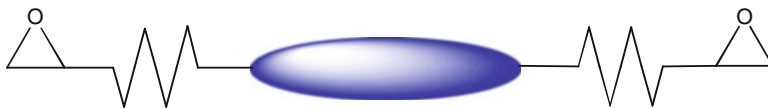
Fig. 1.1 Typical chemical structure of LC epoxy monomers, with a rigid mesogen core, alkyl flexible spacers, and epoxy functional groups on the ends
