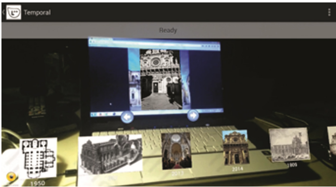
Fig. 2. Result shows an added images slider, on the bottom of the display, and a historical image overlapped on the real scene
