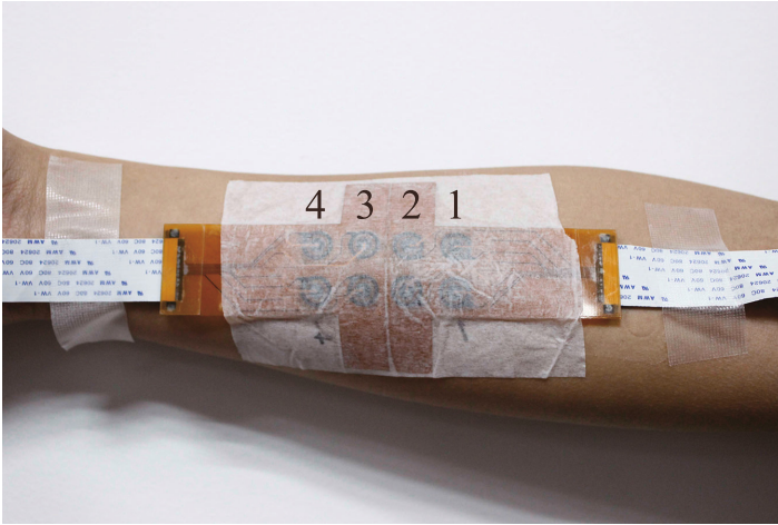
Fig. 2. The multichannel electrodes. Each number represents a channel and each channel is independent. The upper copper pad is anode and the corresponding lower pad is cathode. All of the copper pads are covered with hydrogel to avoid the pricking caused by bad contact between electrodes and skin.
