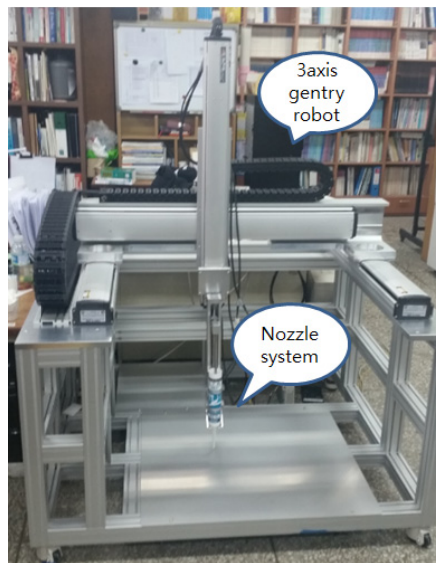
Fig. 2. 3D print for building system
