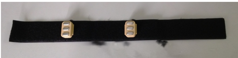
Fig. 3. The EMG acquisition device
