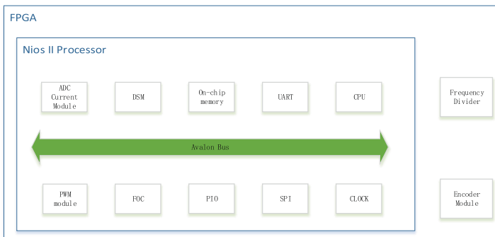
Fig. 2. The structure of SoPC system
