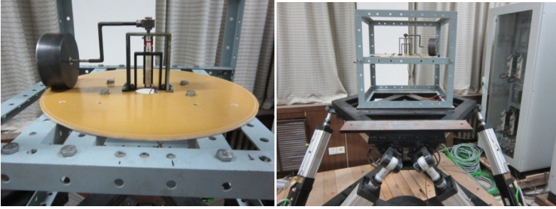
Fig. 6. Six-degree-of-freedom shaking platform
