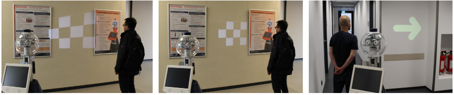
Fig. 6. Example image for the wall segment extraction and projection rectification. left: unmodified and distorted projection. middle: projection after segment extraction and rectification. right: direction information displayed on the wall.
