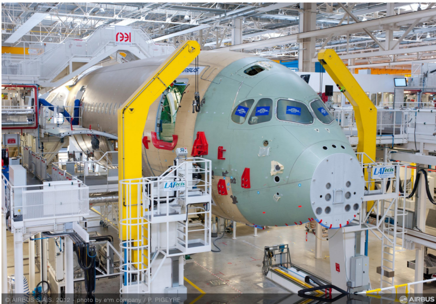
Fig. 1. Airbus A350 XWB first front fuselage in final assembly line in Toulouse, France (source: http://www.airbus.com/galleries/photo-gallery/ )
