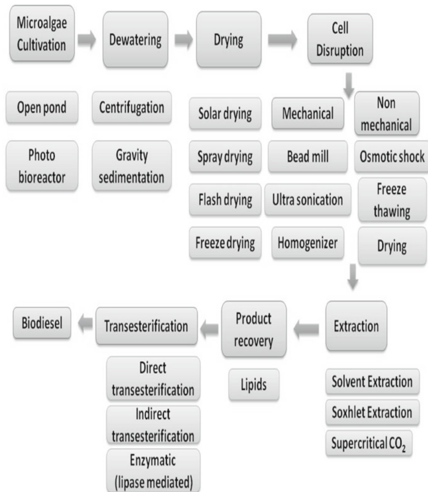
Fig. 15.1 Flow diagram of different unit operations during downstream processing of microalgae.
