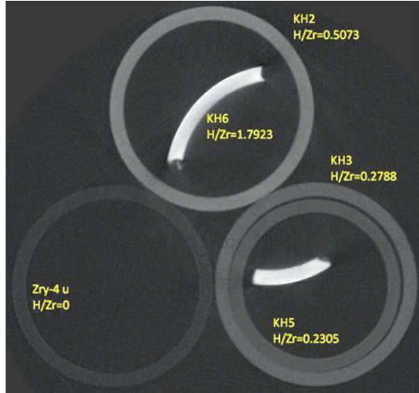
Fig. 7.20 Horizontal slice of the 3D reconstruction of the calibration specimen assembly
