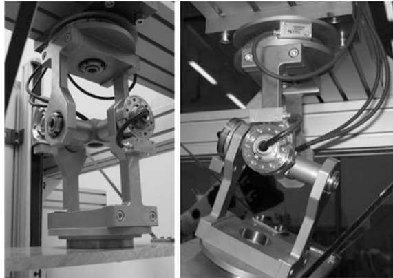
Fig. 3 Three axes Cardan joint in laboratory
