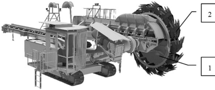
Fig. 1 Compact bucket wheel excavator K100 (NOEN Inc.) (1 – bucket wheel, 2 – bucket)
