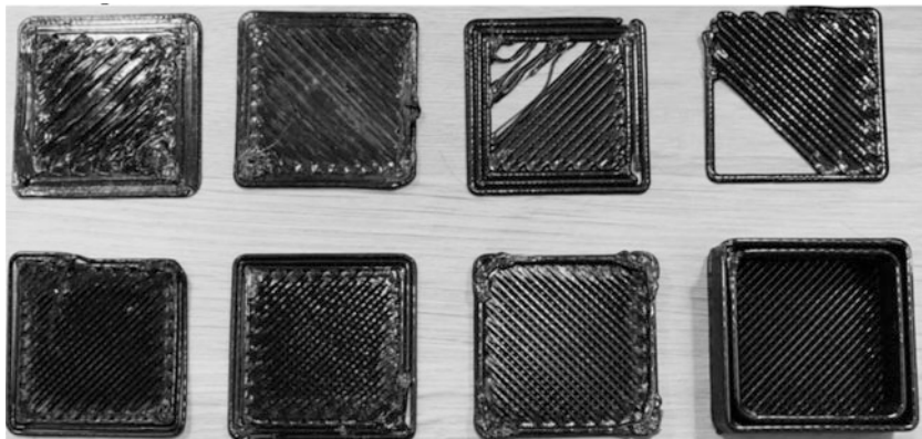
Fig. 2 Same parts printed with different first layer heights and nozzle temperature
