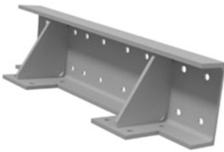
Fig. 5 (a) The frame for attachment of bearing; (b) the arm; (c) the frame for attachment for hydraulic cylinder
