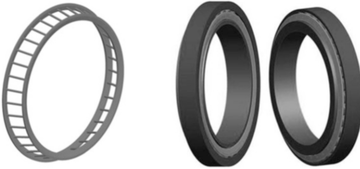
Fig. 1 Tapered roller bearing model in Pro/Engineer
