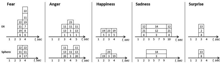
Fig. 2. The combination of design parameters for the emotional expressions of fear, anger, happiness, sadness and surprise, as implemented in a more expressive E4 robot (top) and a less expressive Sphero robot (bottom).
