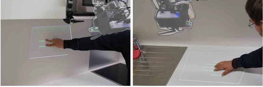
Fig. 5. Touch interaction using the UbiBeam system (UbiBeam is highlighted for better viewability).
