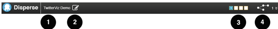
Fig. 5. The Disperse interface appears as a header in each browser window and includes (1) the name of the visualization that is being run, (2) a source code editor, (3) the screen layout, and (4) a branch selector (Color figure online).
