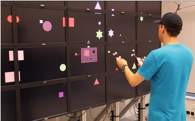
Fig. 1. Test application to evaluate distance-aware manipulation technique with a large high-resolution display.
