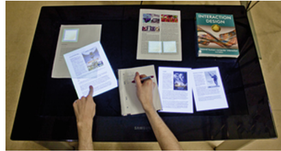
Fig. 1. ProjecTop system visualizing the occluded digital objects
