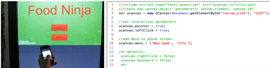
Fig. 4. Left: User connects to uCanvas by entering the canvas’ URL. Right: Adding interactivity to the UI on the left by adding a few lines of Javascript: defining a pointer, a left-click button and a menu.
