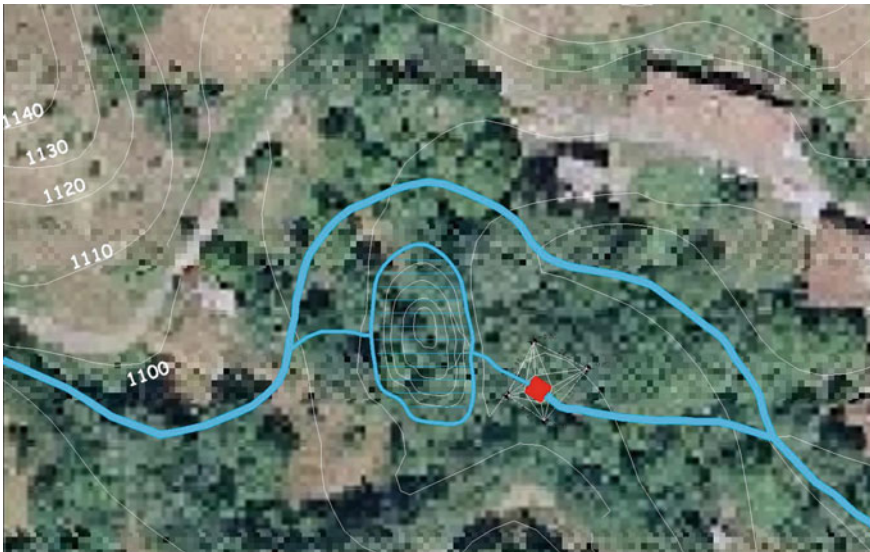
Fig. 5 Hydraulic works of the Fioli mill: the diversion channel and the storage reservoir
