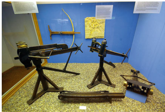
Fig. 16 Catapults in the Saalberg Museum built by Erwin Schramm some time before 1904. Standing on the left is Dionysius’s repeating catapult with sprocket chain. The chain is shown once more at the bottom. Source http://en.wikipedia.org/wiki/Polybolos
