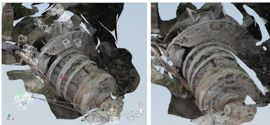
Fig. 16 Photogrammetric three-dimensional reconstruction of the vertical wheel and camshaft for copper processing in Villa Tordinia mill. The reconstruction was realized with the software Autodesk 123D Catch
