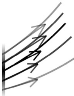
Fig. 1.2 FIVP using \hat{D} -derivative: the solution is a fuzzy bunch of functions X(\cdot) \in \mathcal{F}(E([a, b]; \mathbb{R})) and F is a fuzzy-set-valued function such that F : [a, b] \times \mathcal{F}(\mathbb{R}) \rightarrow \mathcal{F}(\mathbb{R})
