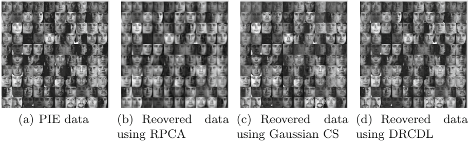
Fig. 1. From (b) to (d), recovering the reduced data from d = 16 , using RPCA, Gaussian CS, and DRCDL, respectively. The PSNR is 23.01 dB, 25.28 dB and 31.12 dB.
