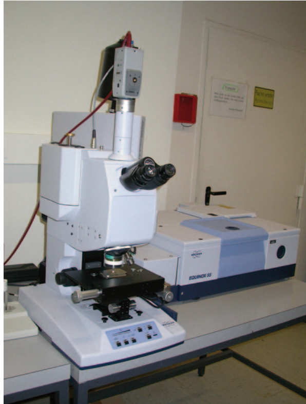
Fig. 4.1 Fourier transform infrared (FTIR) microscope Hyperion 3000 (Bruker Optics, Ettlingen, Germany) equipped with a single-channel detector and a 64 \times 64 focal plane array (FPA) detector
