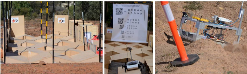
Fig. 2. (Left to right) Continuous 15° pitch/roll ramps; Far-field acuity test; Rover traversing irregular terrain
