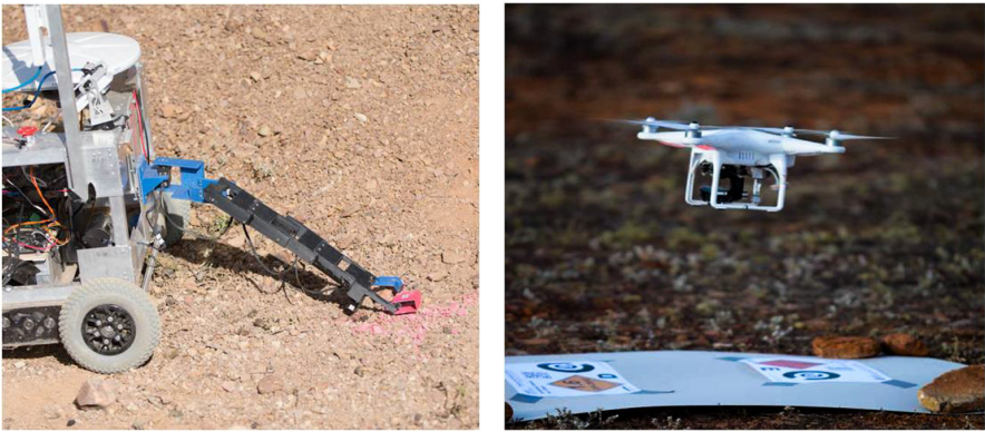
Fig. 4. UNSW Rover collecting the target object during Sample Return task (left). Phantom 2 quadrotor above horizontal visual targets (right).
