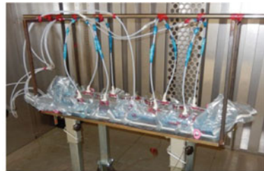
Resin infusion and curing process
