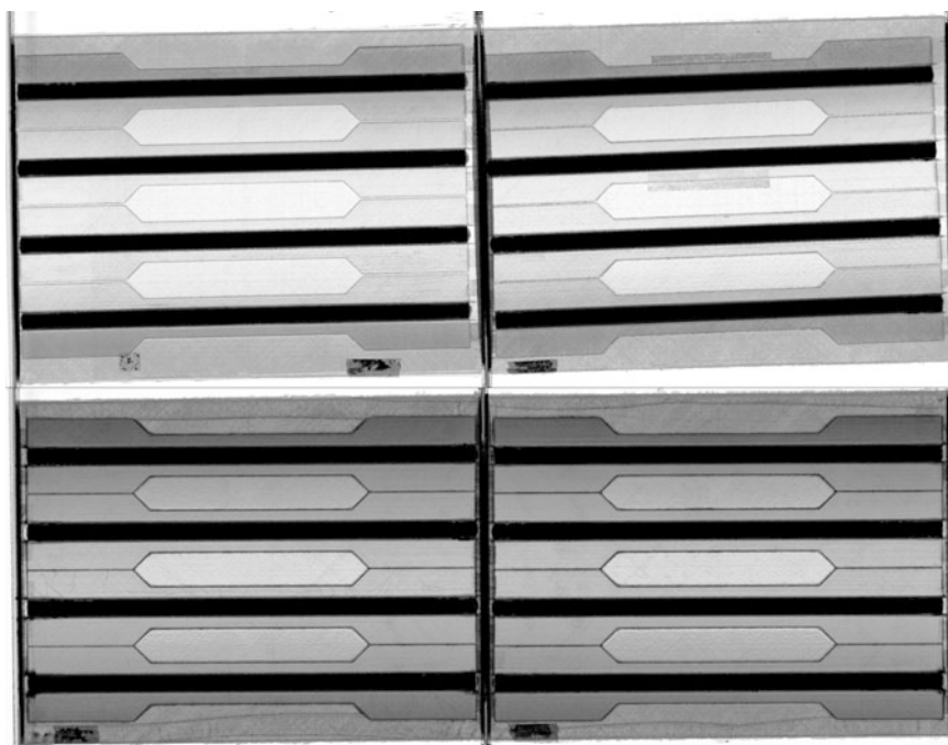
Fig. 18 Batch 1 C-scan top thin (nr 1 left) bottom thick (nr 1 left)
