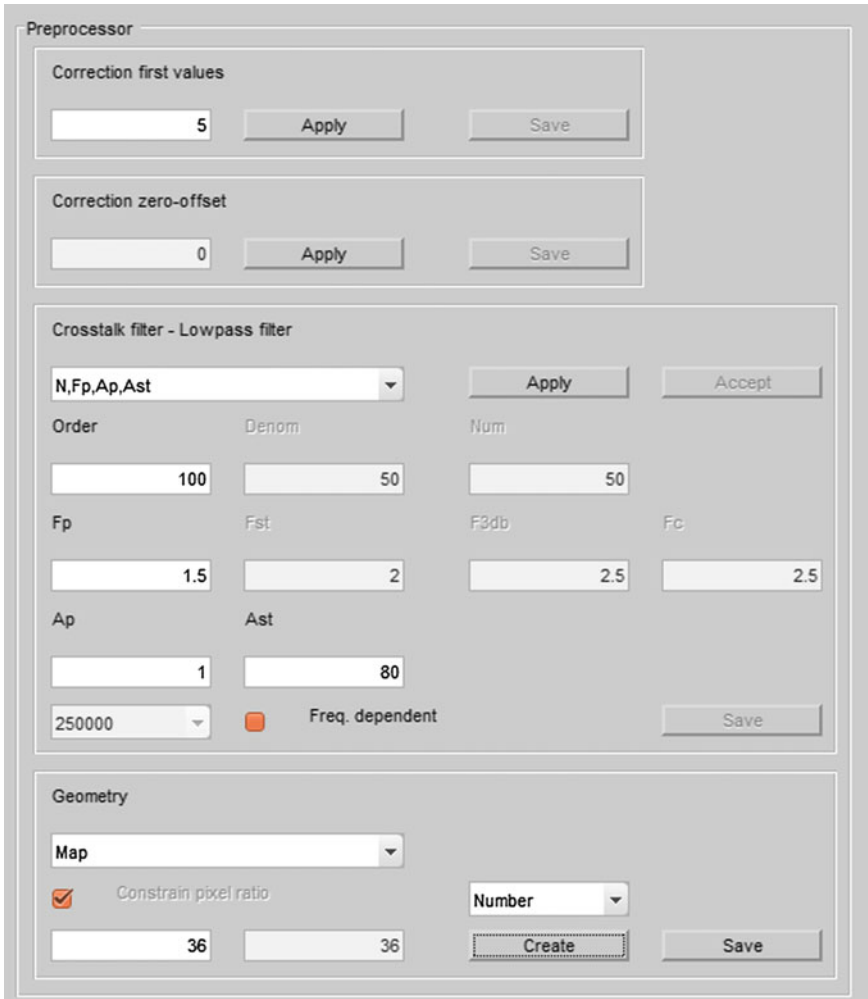
Fig. 4 Preprocessor panel. The signal processing steps are defined in the three sections on the top of the panel, whereas the creation of the grid for mapping the damage intensity is controlled in the bottom section of the panel
