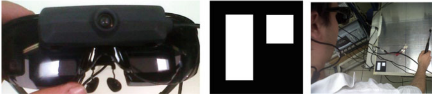
Fig. 10 (Left) Vuzix STAR 1200 glasses used in the research, (center) marker features, (right) image of aluminum sheet with impact marker
