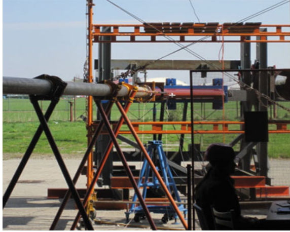
Fig. 13 Bird strike test at VZLU with EADN and conventional aluminium splitter (INVENT)
