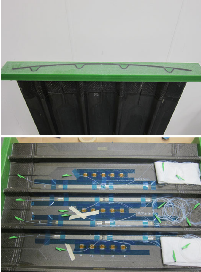
Fig. 16 Machined potting and panel with structural health monitoring sensors
