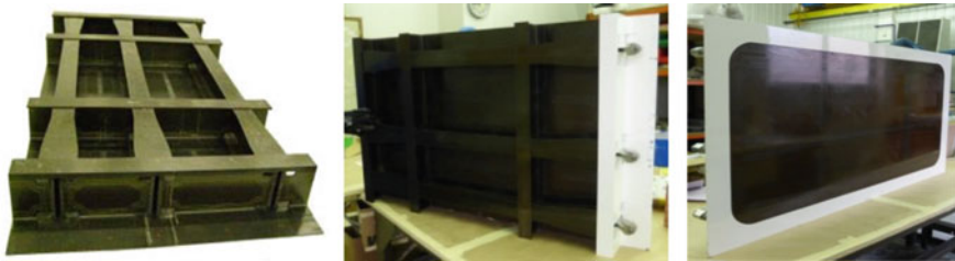
Fig. 11 Left Mini-door after resin transfer moulding (inner surface, unpainted). Middle Mini-door (inner surface, painted). Right Mini-door (outer surface, painted) [2]
