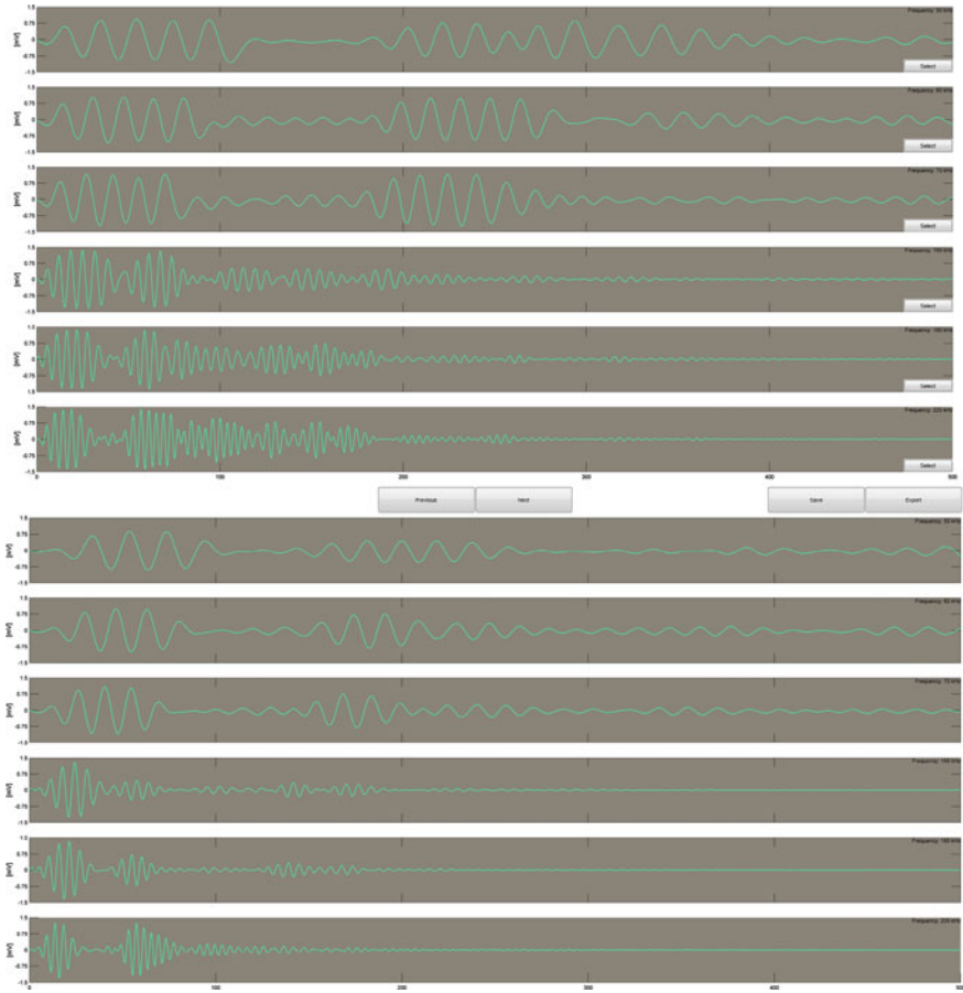
Fig. 2 Waveforms at different frequencies between two pair of sensors ( top parallel to stringer, bottom across stringer)
