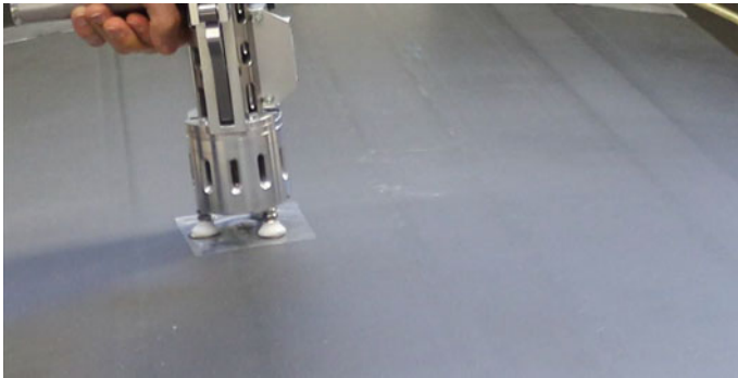
Fig. 7 Introduction of impact at CFRP panel (structure representative to door surround panel)
