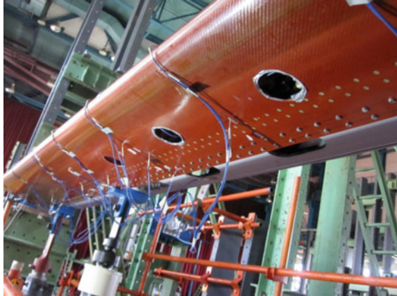
Fig. 14 Additionally fitted access holes for fast kinematics repair in the test setup (INVENT)
