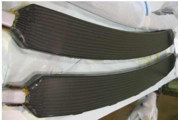
Fig. 6 Cured preform after extraction from mould
