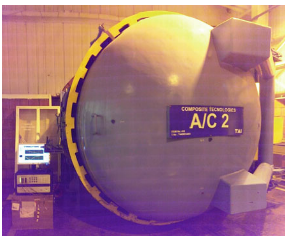
Fig. 12 Thermal profile identification—trial autoclave run with the skin tool
