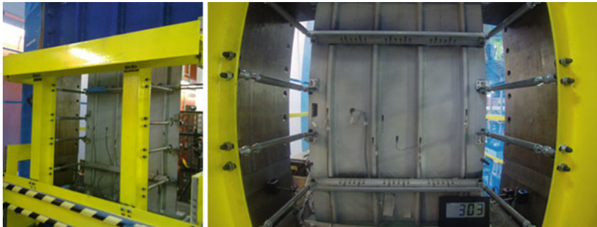
Fig. 4 Designed framework to provide out-of-plane support to the panel
