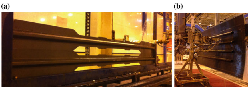
Fig. 21 Ultrasonic inspection of components— a Stringer inspection. b Lower panel inspection
