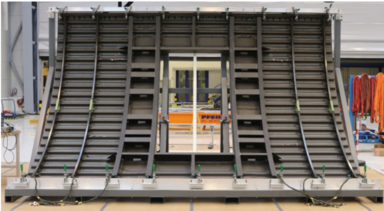
Fig. 6 The completed door surround structure panel in its dual purpose transportation and testing rig
