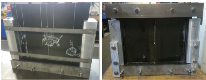
Fig. 8 Installation of anti-buckling guide to panel ( front and back )
