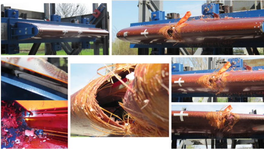
Fig. 17 Experimental test results on specimen 3/BSPS splitter 3 installed in a representative morphing leading edge
