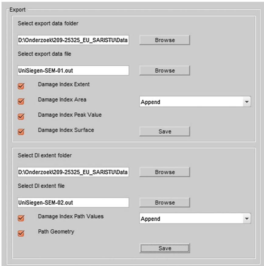
Fig. 7 Export panel. Two different output files, both in ASCII format, can be exported. The content of the files can be adapted by (de)activating the checkboxes
