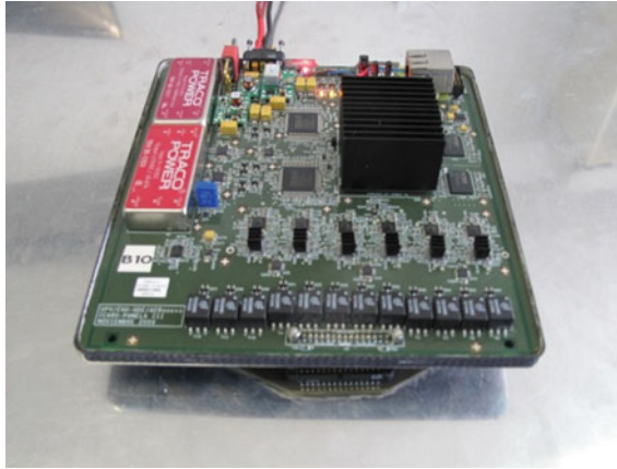
Fig. 1 The PAMELA III with all electronic components inside the composite box placed over the PhA transducer adapter and bonded to the structure to perform SHM testing
