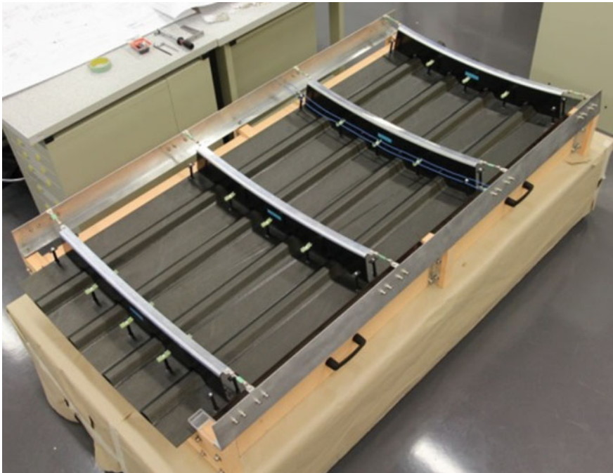
Fig. 13 Side panel assembled into its electrical testing rig [11]
