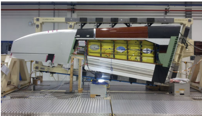
Fig. 12 SARISTU morphing wing consists of different morphing devices which functionality will be tested in a wind tunnel test at TsAGI, Moscow
