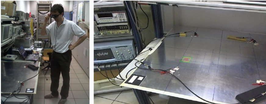
Fig. 12 Experimented with AR glasses ( left ) and image visualized by the experimenter with a virtual marker over imposed to the structure ( right )
