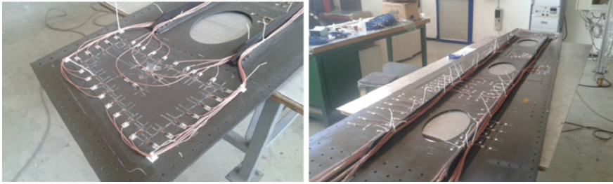
Fig. 22 Cabling implementation on the lower wing panel. a group A and b overall view
