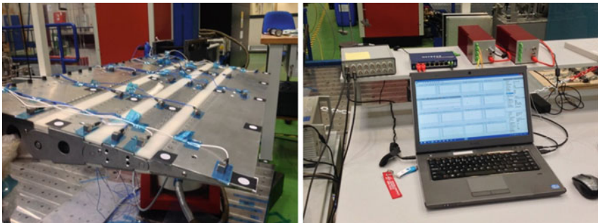
Fig. 21 Test setup for the 2-bay ATED demonstrator
