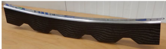
Fig. 24 Resin infusion process and cured part after machining to final contour
