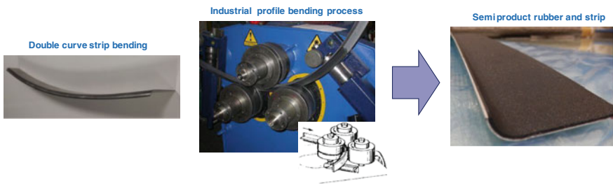
Fig. 2 Semi-product manufacturing process
