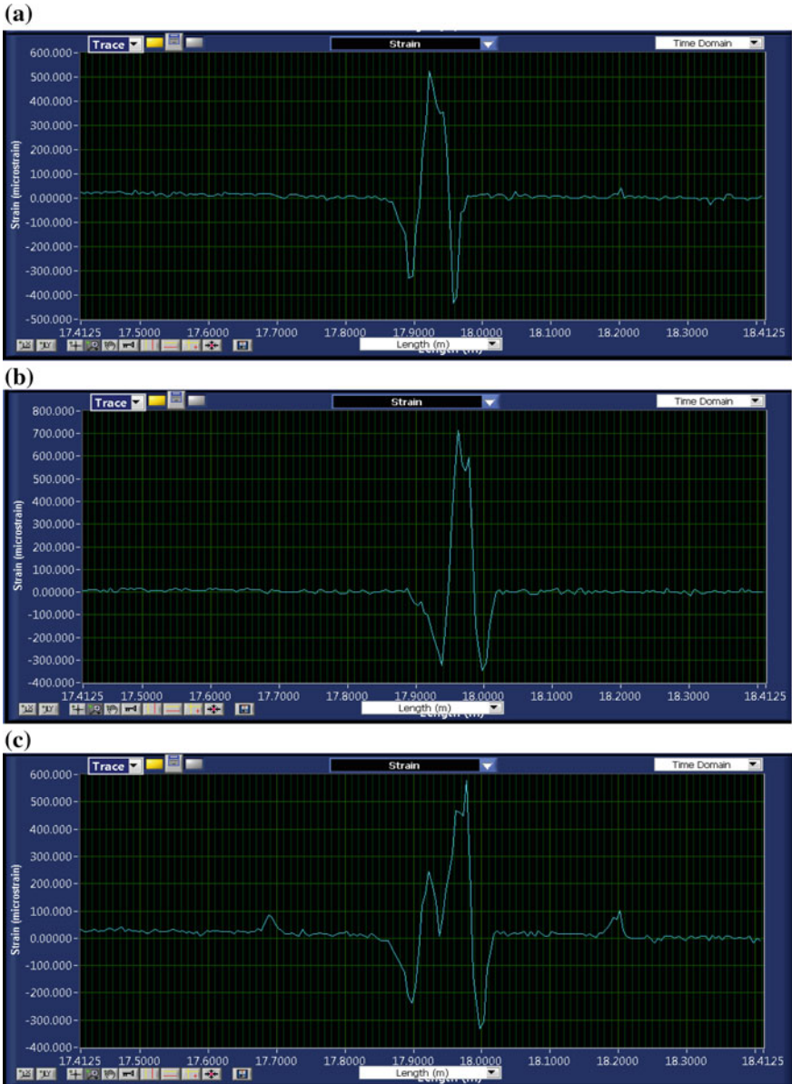
Fig. 19 Distributed measurement of the strain following impacts. a After one impact; b after 2 impacts, spaced 40 mm apart; c after two impacts, but references to the panel state before the first impact
