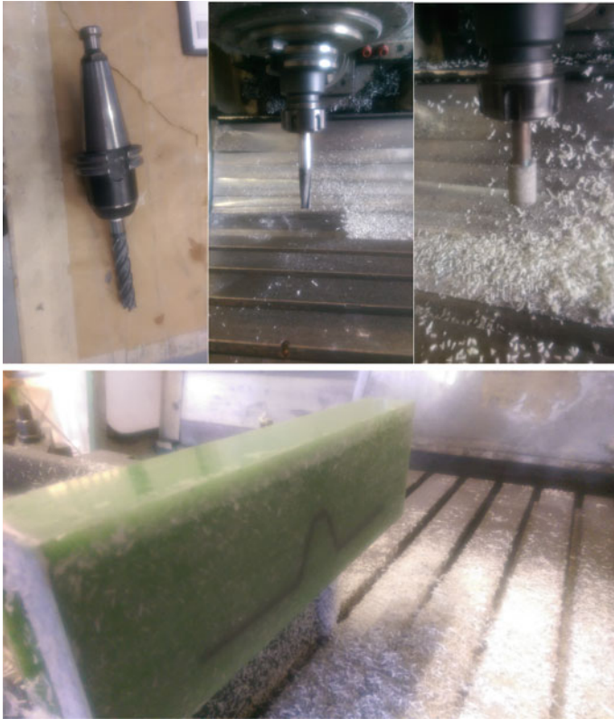
Fig. 15 Machining of potted panel tests of end mill type
