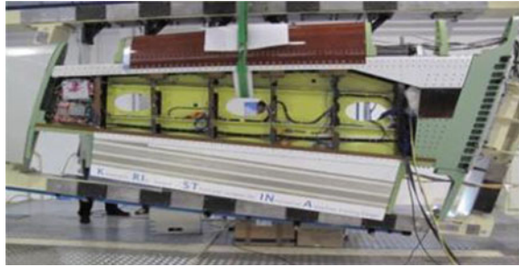
Fig. 13 Assembly of leading edge to the wing section
