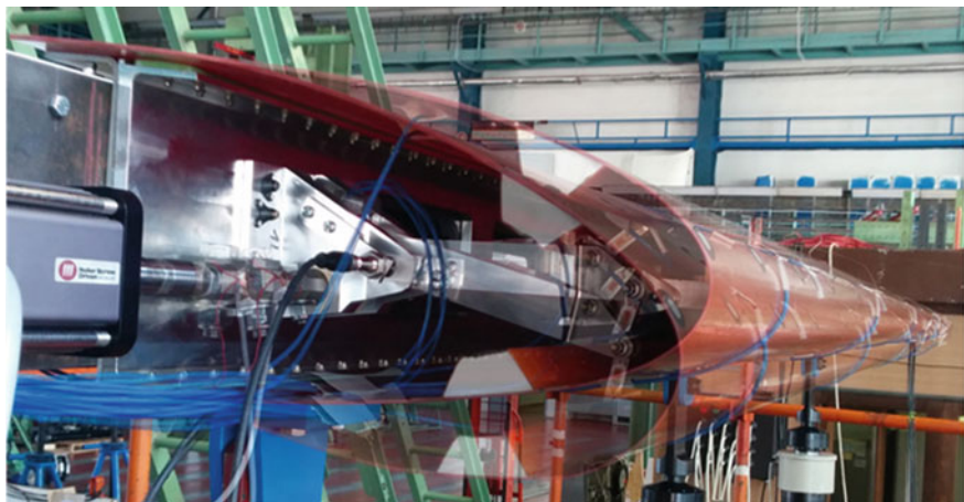
Fig. 17 Fully integrated droop nose at VZLU during life cycle ground test
