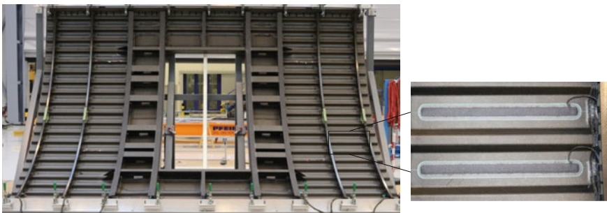
Fig. 7 Manufactured door surround structure with integrated SHM network
