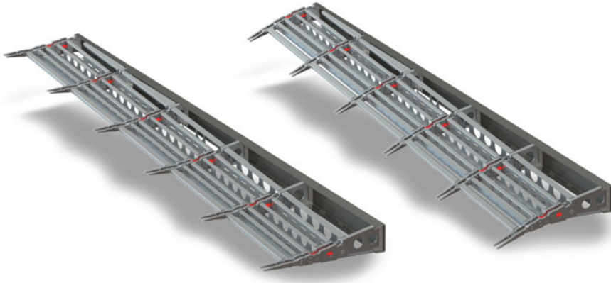
Fig. 4 ATE configuration: morphed up ( left hand side ), morphed down ( right hand side )
