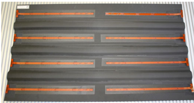
Fig. 2 Stiffened composite structure with 40 cobonded piezoelectric SMARTLayer ® transducers
