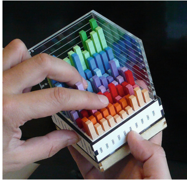
Fig. 1. A physical three-dimensional bar chart made of laser-cut acrylic automatically generated from data. Each bar was spray-painted and mounted on a base together with two scales made from transparent acrylic sheets on which axis labels and lines were engraved. Country and year labels were engraved on all four sides of the base using a vertical orientation.
