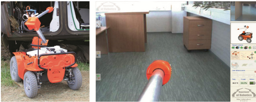
Fig. 1. Mobile robot Hercules and a screenshot of its existing graphical 2D user interface
