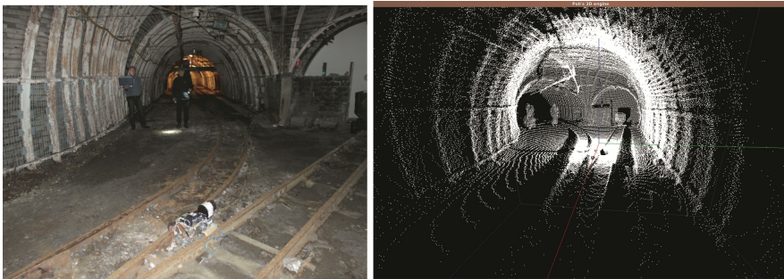
Fig. 2. Photo of the turning in the Coal mine and 3D view on the turning surroundings
