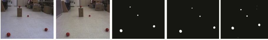
Fig. 6. The images of first target for the verification of the data fusion accuracy: the left and right CCD cameras (left); the left and right thermal imager cameras (center); the TOF camera intensity image (right).
