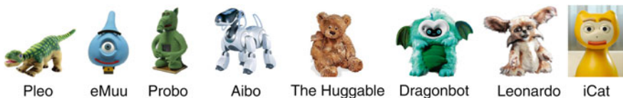
Fig. 3 Pet robots (from left to right ): Pleo, eMuu, Probo, Aibo, The Huggable, Dragonbot, Leonardo, iCat
