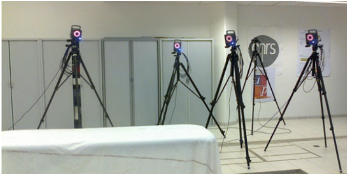
Fig. 2 Experimental setup: cameras of the Vicon Nexus motion capture system
