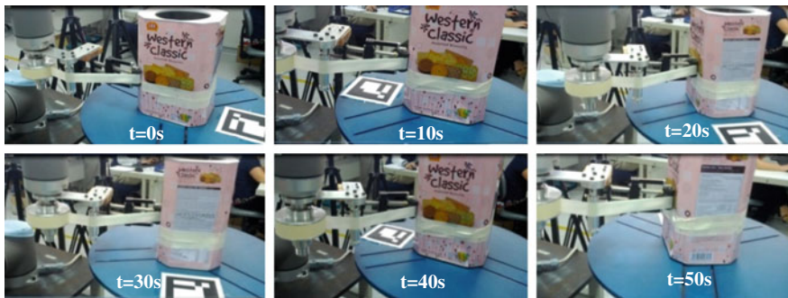
Fig. 6 Snapshots of experimental test for an automated robot taping
