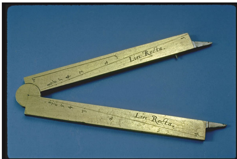
Fig. 1 Rectilinear line (proportional scale) on Italian-style sector, early seventeenth century. Catalog number 321678. Negative number 74-1250. Courtesy of the Mathematics Collections, Division of Medicine & Science, National Museum of American History, Smithsonian Institution
