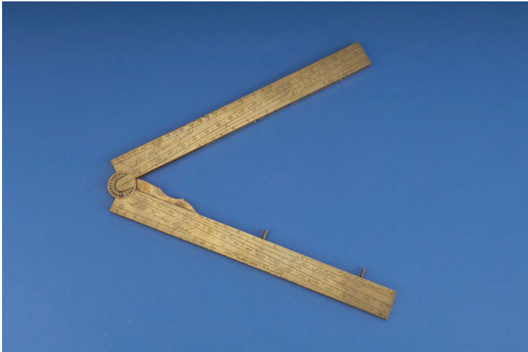
Fig. 3 French-style sector, eighteenth century. Scales shown are poids des boulets , line of lines, line of solids, and tetragonic line. Cat. no. 314799. Neg. no. DOR2012-2585. Courtesy of the Mathematics Collections, Division of Medicine & Science, National Museum of American History, Smithsonian Institution
