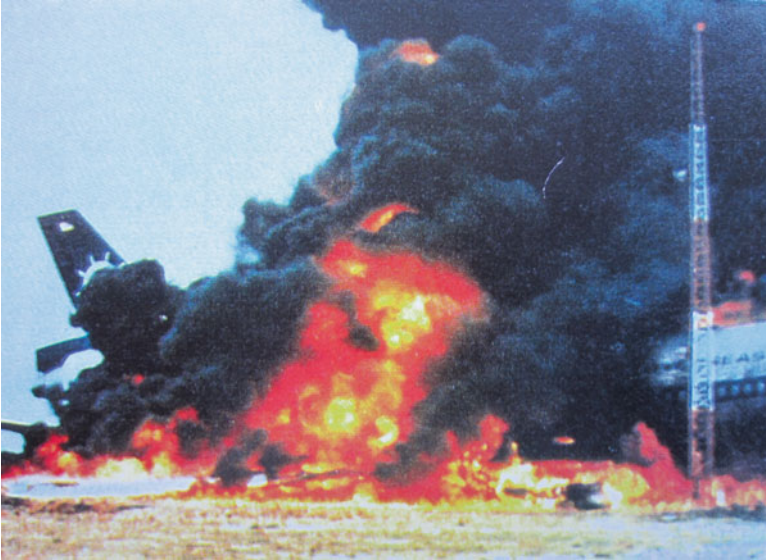
Fig. 21.3 The DC10 burning fiercely after an engine disintegrated as the result of an engine ingested a number of the larger varieties of Gulls ( Larus sp.). All 139 on board escaped (photo Port of New York Authority)
