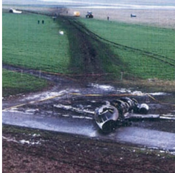
Fig. 21.5 The remains of the Falcon 20 which attempted to force land at Paris Le Bourget after an engine disintegrated during take-off rupturing a fuel tank and setting the aircraft on fire. All 10 on board were killed. 15 dead Lapwings ( Vanellus vanellus , 215 g) were found on the runway (photo BEA Report f-In950120)
