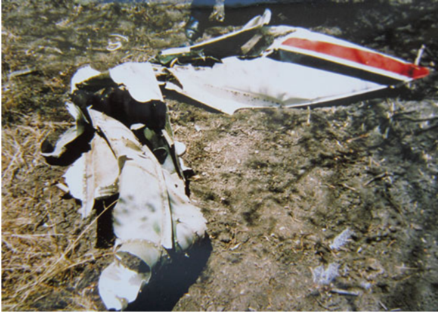
Fig. 21.8 The Cessna 402 wing tip and aileron together with part of the Marabou Stork ( Lepoptilos crumeniferus , 5.9 kg) embedded in it. All seven on board were killed after the pilot was unable to maintain control (photo via J Thorpe)
