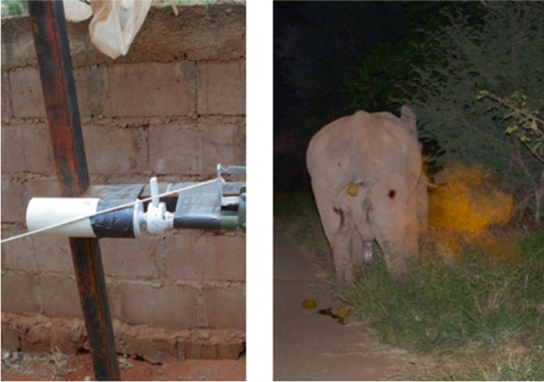
Fig. 7.9 The two types of EL@OUT in action: while the manual version is peppering an undesirable individual, the automatic version will be triggered by the elephant itself when entering in the no-go area © S Le Bel © PPP
