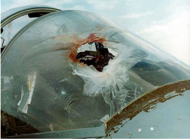
Fig. 21.13 Typical damage to the windshield of a military fast jet following impact with a bird which has the same effect as a bullet (photo via J. Thorpe)
