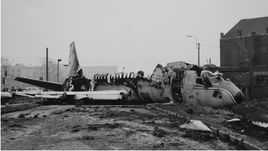
Fig. 21.4 The wreckage of the Boeing 737 at Gossellies, Belgium, after a single Woodpigeon ( Columba palumbus , 465 g) was ingested by an engine. The three crew escaped (photo via J Thorpe)
