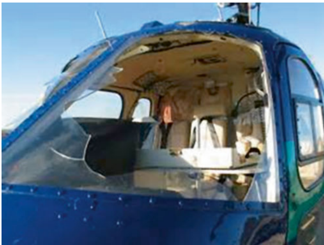
Fig. 21.12 A typical case of a shattered helicopter windshield (photo via J. Thorpe)
