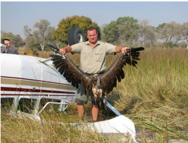
Fig. 21.10 This African white-backed vulture ( Gyps africanus , 1.7 kg) smashed through the windshield of the Cessna 206 while it was flying at 2500 ft over The Okavango nature reserve in Botswana. The pilot and four passengers escaped with minor injuries (photo via J Thorpe)
