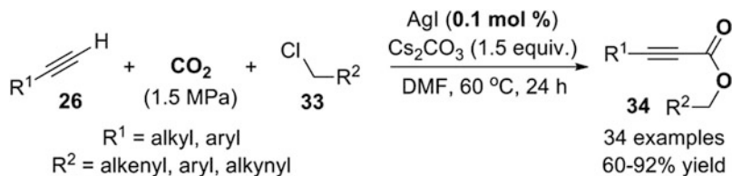
Scheme 21 Silver-catalyzed carboxylative coupling reaction of the terminal alkynes, carbon dioxide, and chloride compounds
