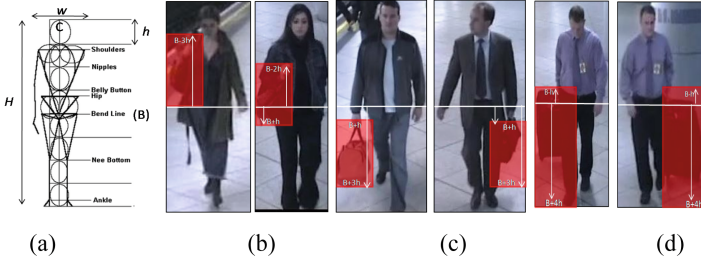
Fig. 1. Human-baggage spatial model of front view direction. The category of bag is divided into three major categories according to body proportions (a); (b) backpack or hand bag, (c) tote or duffle bag, and (d) rolling luggage.
