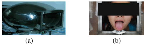
Fig. 2. (a) Tongue image acquisition device. (b) Original image.
