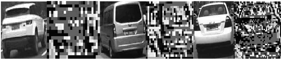
Fig. 1. The MB-LBP feature images of the vehicle
