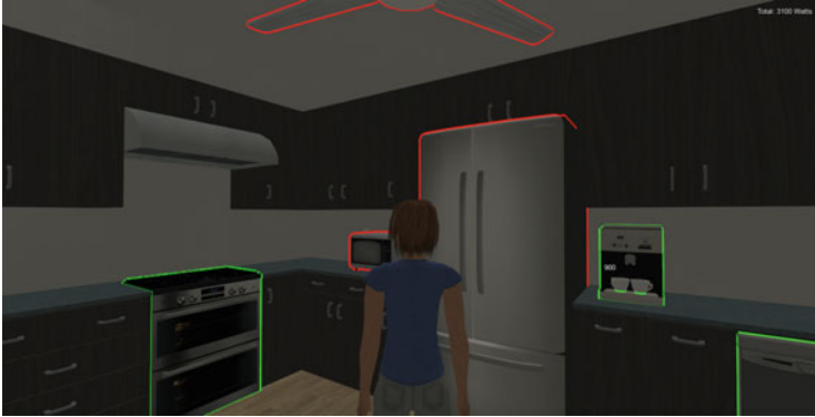
Fig. 5 The coffee maker is “on” as denoted by the green outline, and the number 900 superimposed over it indicates that it is consuming 900 W of power. The 3100 W in the upper-right corner is the total wattage of the coffee maker, stove, and dishwasher
