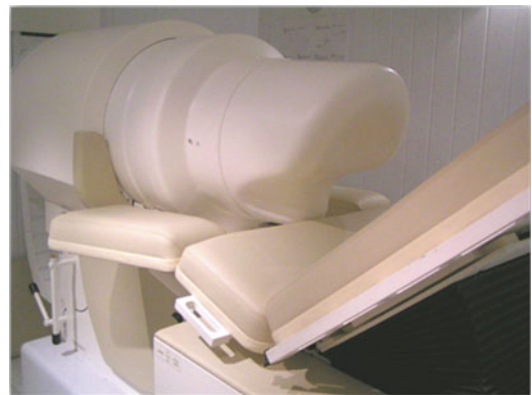
Fig. 23.1 Dedicated fetal biomagnetometer with maternal support. Women are seated in a slightly reclined position with legs on both sides of the biomagnetometer interface. The concave surface of the sensor array overlays the gravid maternal abdomen
