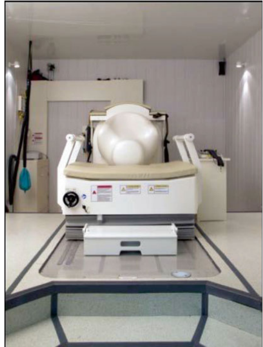
Fig. 22.1 SARA II System (SQUID Array for Reproductive Assessment, VSM MedTech Ltd., Port Coquitlam, Canada) installed at the fMEG Center in Tübingen
