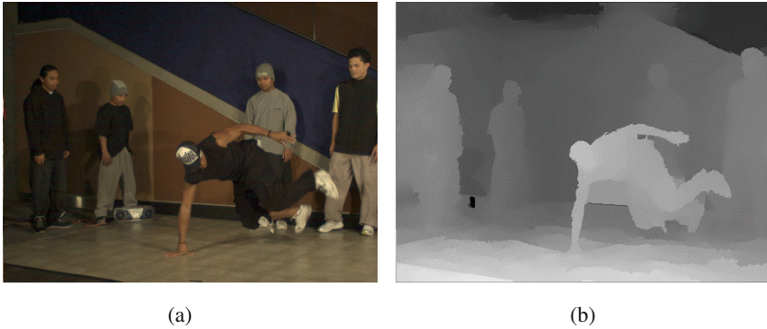
Fig. 1. The video plus depth format of 3D video: (a) the texture video; (b) the depth map.
