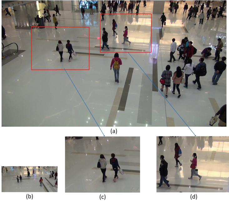
Fig. 3. (a) is the frame from the PTZ camera panorama view; (b) is the frame from the static camera view; (c) is the view generated from (a) with the virtual PTZ camera at parameters (pan:7.62, tilt:-2.17, focal length:4500); (d) is the view generated from (a) with the virtual PTZ camera at parameters (pan:-1.68, tilt:-4.37, focal length:5000)
