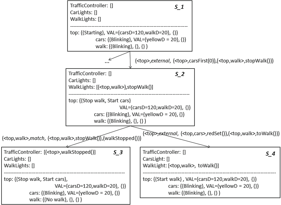
Fig. 9. Execution states of the UML-RT model (Figs. 2, 3 and 4) using state aggregation abstraction. We assume that toRed is external signal.
