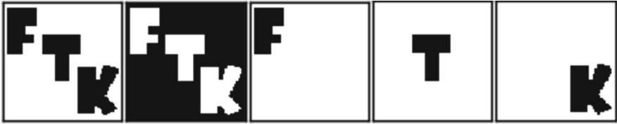
Fig. 2. Initial image 'FTK' at the left and then allocated segments from the image where back masks represent allocated objects: background, letter 'F', letter 'T' and letter 'K' ( \delta_{\text{color}} = 0.12 , \delta_{\text{obj}} = 0.5 ).
