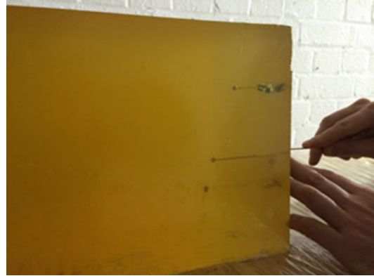
Fig. 11.3 Measuring depth of penetration of 5 mm spherical fragment simulating projectiles fired at a range of velocities into a block of ballistic gelatine
