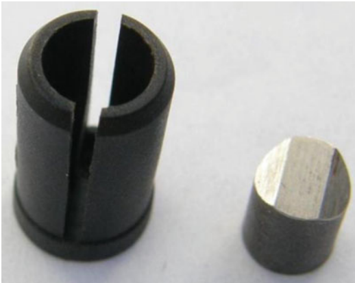
Fig. 18.6 A 1.10 g chisel nosed fragment simulating projectile that can be held within a plastic sabot capable of being fired from a 7.62 barrel
