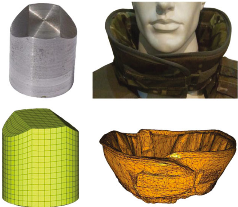
Fig. 27.2 Meshed images of a chisel-nosed cylindrical fragment simulating projectile and the Mark IVa OSPREY half neck collar ( http://www.army.mod.uk/documents/general/20120215-Osprey_Mk4_Instruction_Booklet-R.pdf )
