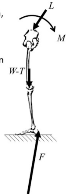
Fig. 2.5 Different free body diagrams under the same blast loading situation at time t = 0 . These demonstrate that the appropriate choice of a free body diagram can allow internal forces to be quantified
