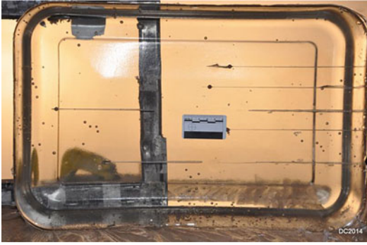
Fig. 11.5 A block of PermaGel™ being used to simulate the penetration of 5 mm spheres: note the physical similarity to gelatin
