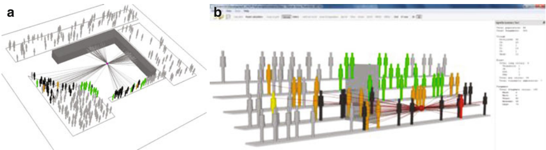
Fig. 17.11 Use of numerical fragment flight algorithms within the HIP code to represent the effect of protective barriers within (a) a tiered, stadium-type environment and (b) a crowded space during an explosive attack
