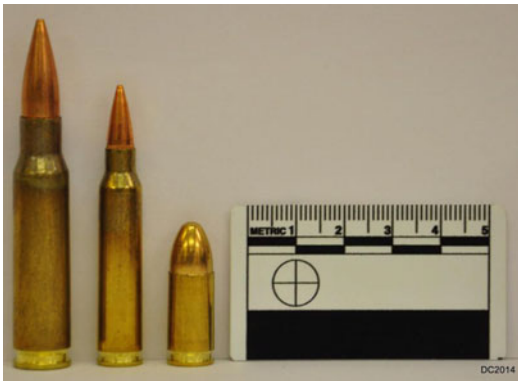
Fig. 18.1 The most common types of bullets utilised on the battlefield (from left to right); 7.62 NATO BALL and 5.56 × 45 mm rifle bullets compared to 9 × 19 mm handgun bullet
