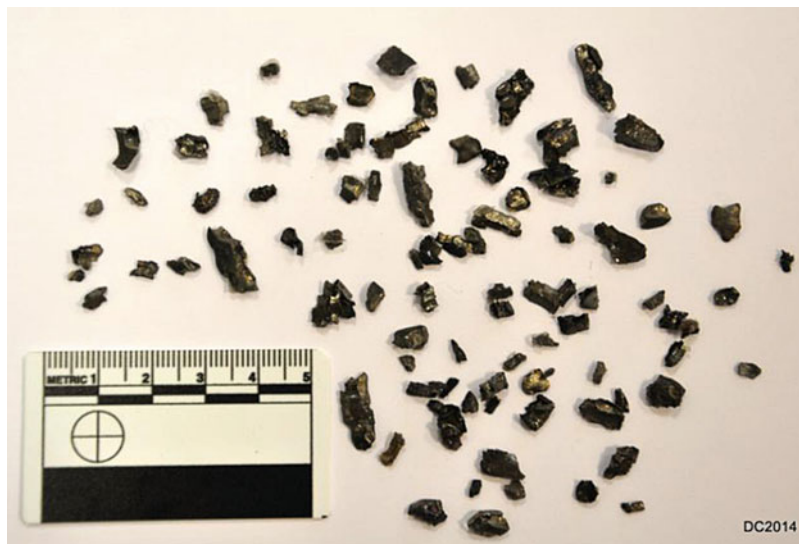
Fig. 18.5 Range of sizes of energised fragments produced by a typical mortar
