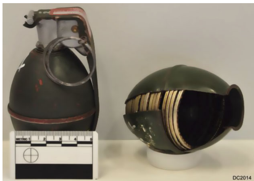
Fig. 18.2 Cross section of a fragmentation grenade in which detonation of the explosive core (not present in this demonstration model) causes the scored steel rings within the case to fragment
