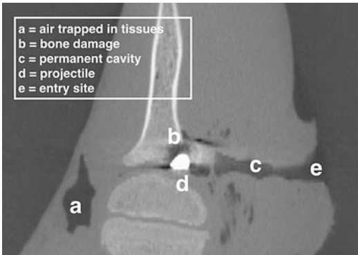
Fig. 11.6 Coronal section of a computed tomography scan following ballistic experimentation using a chisel nosed fragment simulating projectile fired into porcine tissue
