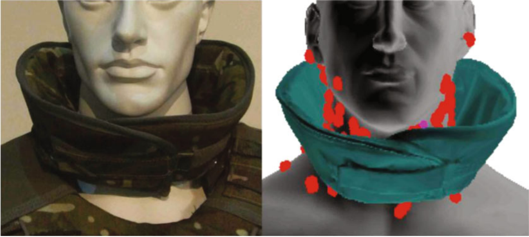
Fig. 27.7 The IMAP Surface Wound Mapping tool demonstrating entry wound locations on the neck of a representative UK male soldier wearing an OSPREY ballistic neck collar
