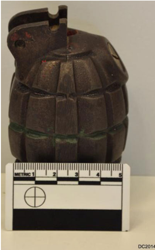
Fig. 18.3 An early style of fragmentation grenade in which the explosive core causes the outer casing to fragment. Originally the casing was grooved to make it easier to grip and not as an aid to fragmentation, and in practice it has been demonstrated that it does not shatter along the segmented lines (natural fragmentation)
