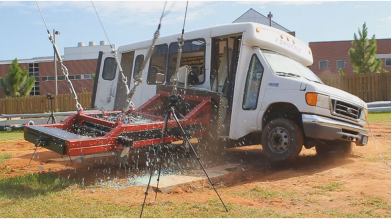
Fig. 23.10 Frame capture from the side impact experiment
