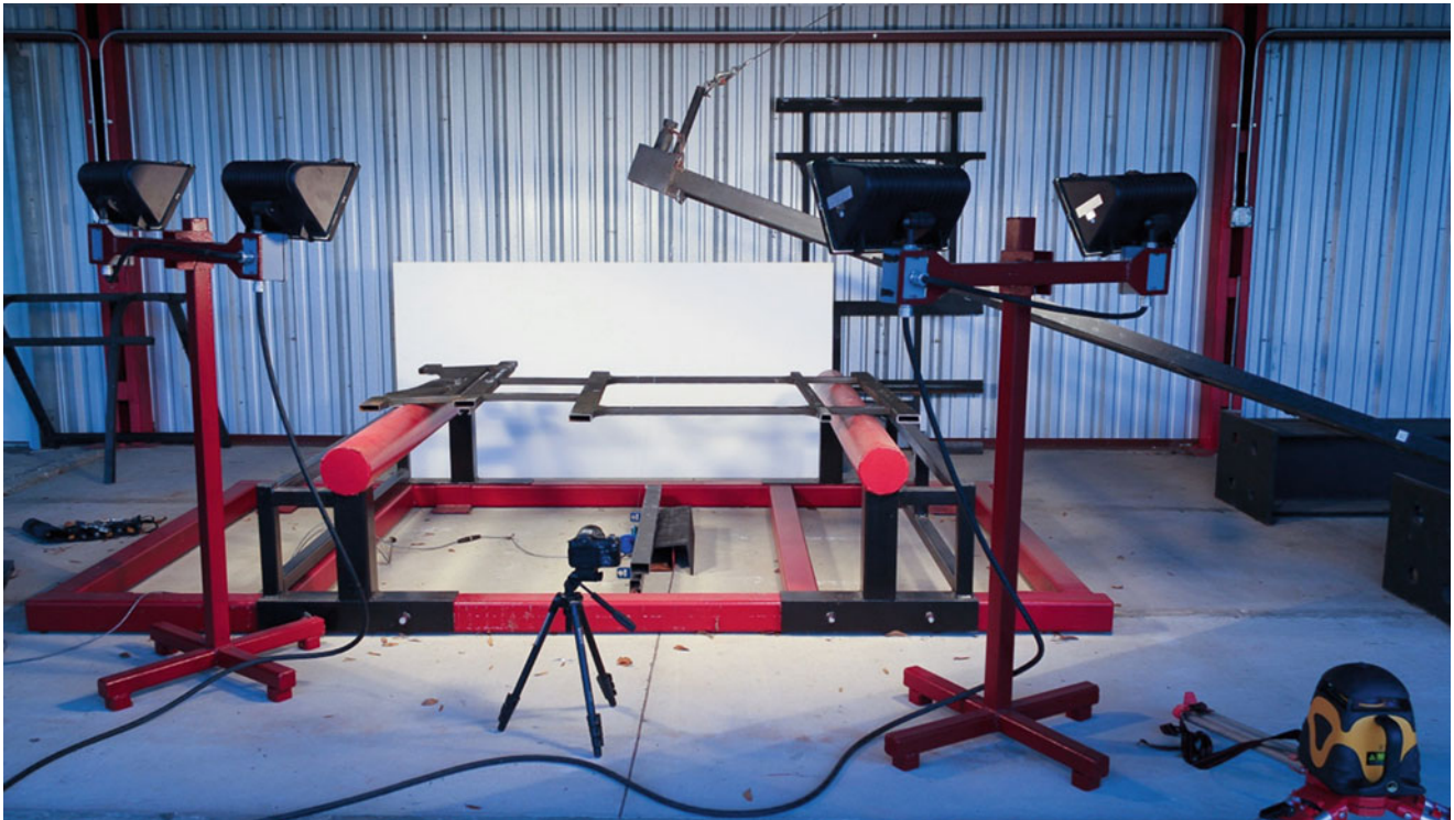
Fig. 23.7 Sidewall panel testing apparatus
