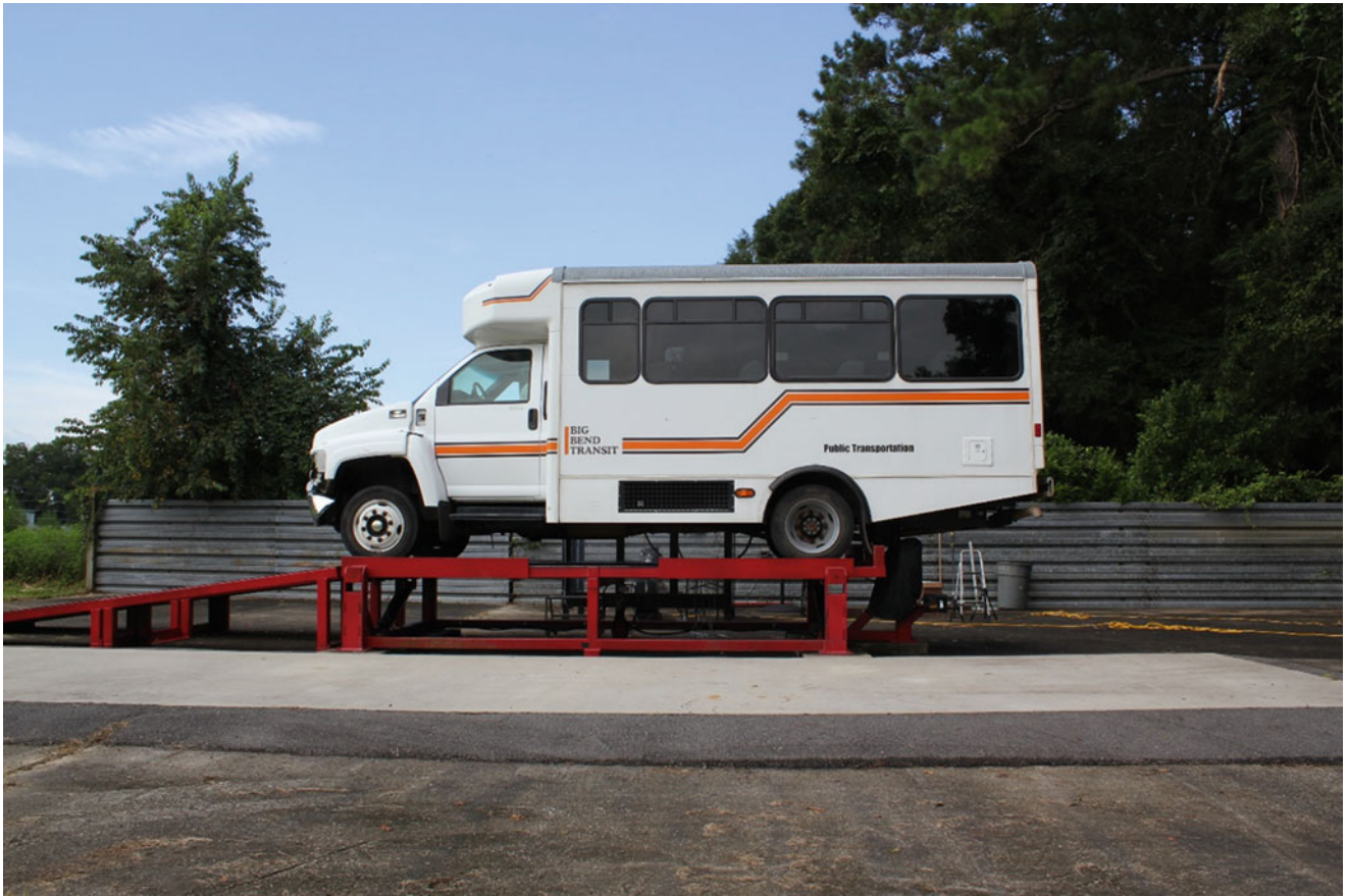
Fig. 23.8 Test setup for the full scale rollover test
