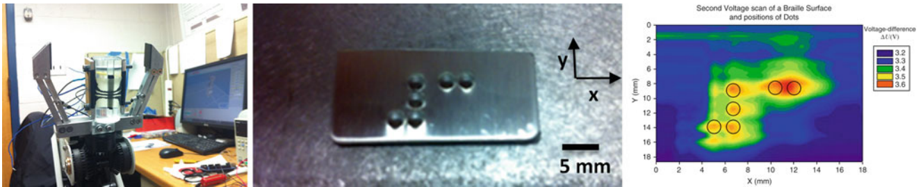
Fig. 4.12 (Left) Finger with sensing skin attached to the robot arm, (center) braille target, and (right) change in voltage from sensing skin raster over Braille target
