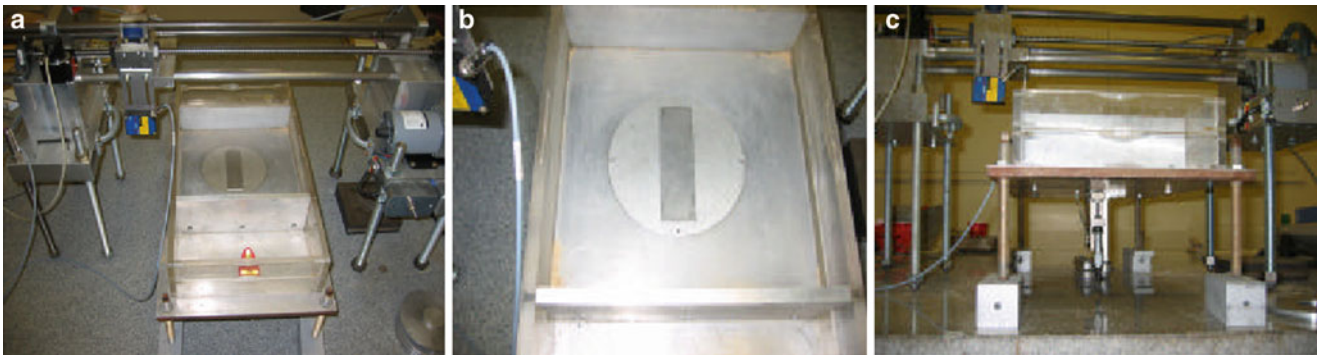
Fig. 41.9 (a) Subsidence cavity model under the surface displacement measurement system; (b) top view; (c) side view
