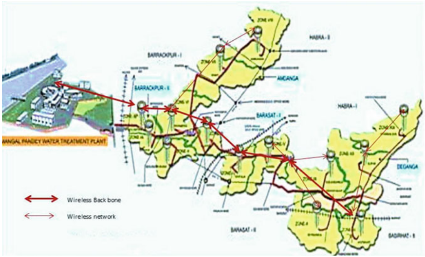
Fig. 8 IoT network in north 24 Pgs Arsenic area water supply scheme
