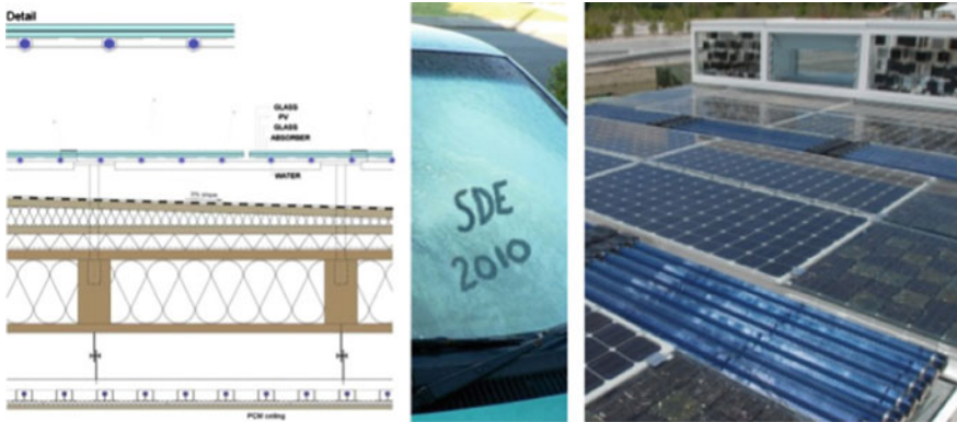
Figs. 5.8–5.10 Principle of PV/T collectors on the roof and PCM ceiling (Source HFT Stuttgart)
