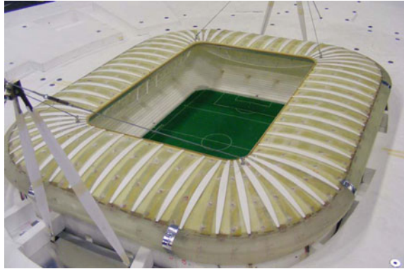
Fig. 2.1 The model of the New Juventus Stadium in Turin tested in the wind tunnel of the Politecnico di Milano ( Source Courtesy Canobbio S.p.A.)
