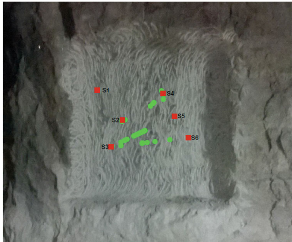
Fig. 21.6 PZT USAM sensors (square) and AE source localization with preferential crack propagation (circle)
