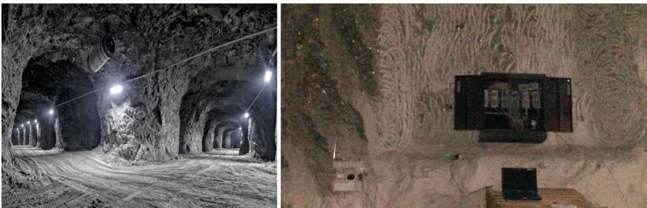
Fig. 21.3 San Pietro Prato Nuovo gypsum quarry ( left ). The six AE devices and the ATOMTEX ^3\text{He} neutron radiation monitor applied to the selected pillar ( right )
