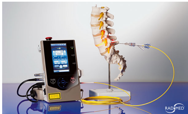
Fig. 6.4 Diode laser 980 nm and laser fiber set, Radimed GmbH
