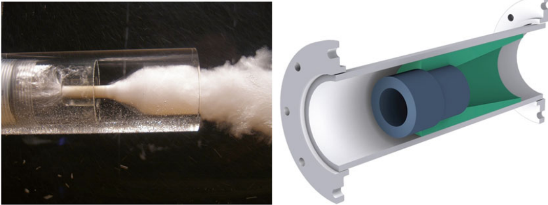
Fig. 2.9 A model of the CavTube™ sparging system (with permission from Eriez)
