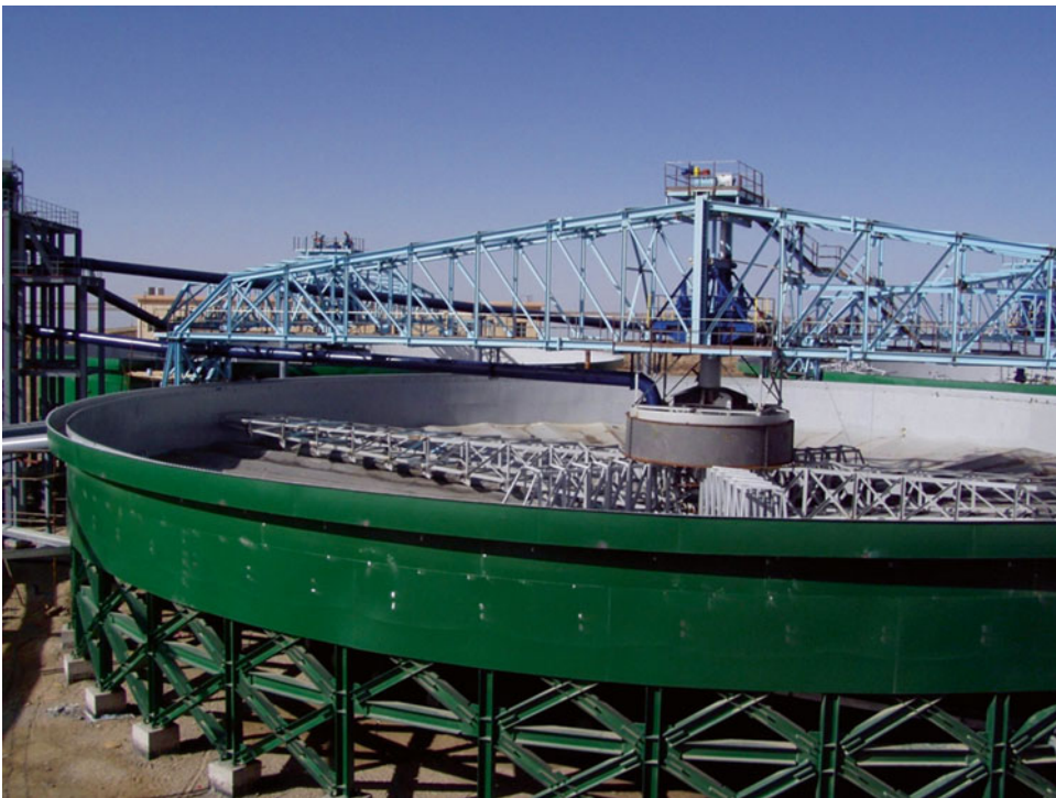
Fig. 12.2 General view of FLS-Dual Drive Thickener. Reproduced with permission from FLSmidth
