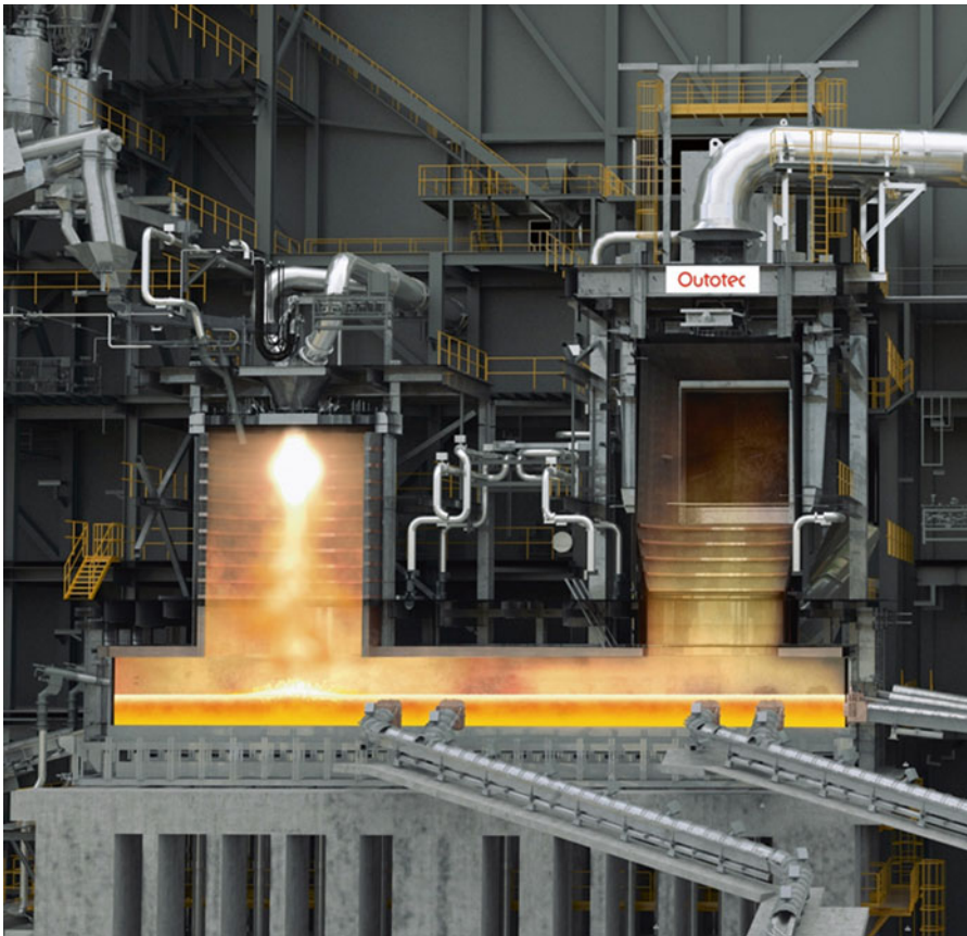
Fig. 16.1 A view of the Outotec flash smelting unit showing feed system, burner, reaction shaft, settler, and uptake. Reproduced with permission from Outotec Inc
