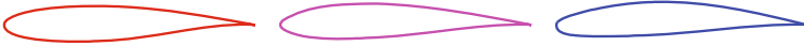
Fig. 3.6 Optimization of a 2D isolated airfoil: three airfoil shapes corresponding to the low lift-low drag part of the Pareto front (first sub-front) shown in Fig. 3.5. From left to right the three airfoils yield the following C_L, C_D values: (0.707, 0.00901), (0.817, 0.00918) and (0.894, 0.00948)
