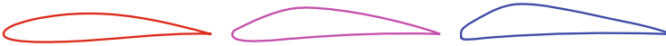
Fig. 3.7 Optimization of a 2D isolated airfoil: three airfoil shapes corresponding to the high lift-high drag part of the Pareto front (second sub-front) shown in Fig. 3.5. From left to right the three airfoils yield the following C_L, C_D values: (0.968, 0.00978), (1.096, 0.010678) and (1.19, 0.01136)
