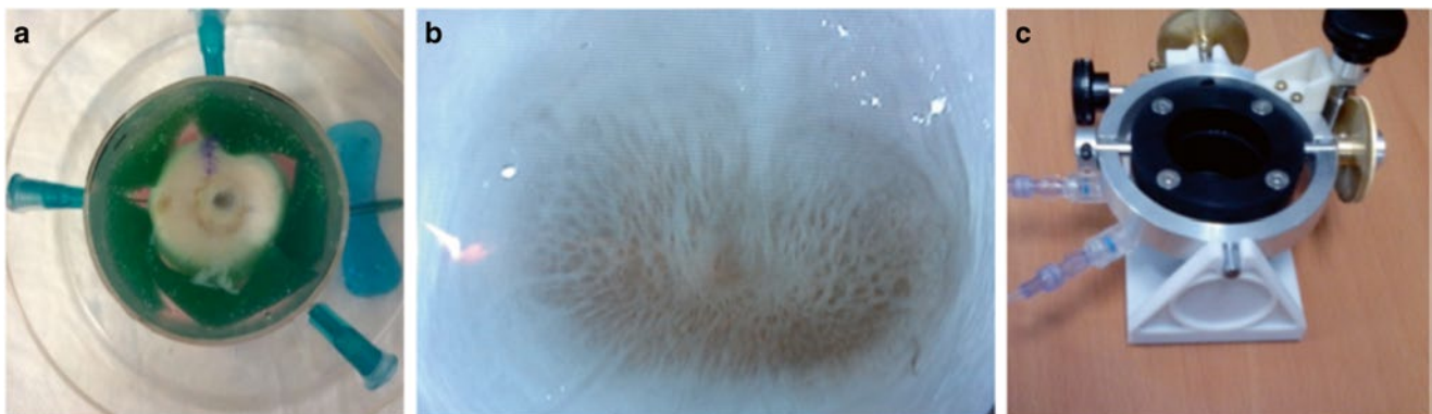
Fig. 2.1 Experimental preparation: (a) Exposed LC of prepared eye, (b) whole-globe human eye holder and (c) posterior sclera holder
