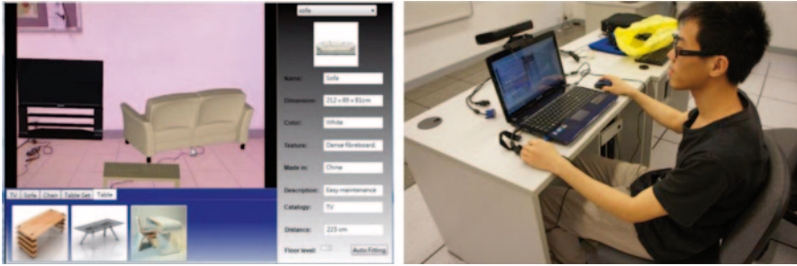
Fig. 27 The user interface of a 3D furniture arrangement system with markerless AR, making use of the microsoft KINECT depth sensor (Tang et al. 2014) ( left ). A user was operating the system ( right )
