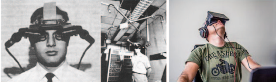
Fig. 19 The world’s first HMD system— The sword of damocles created by Sutherland (1968) ( left ). Head-mounted display in older days ( left ). The rift HMD developed by Oculus VR ( right )
