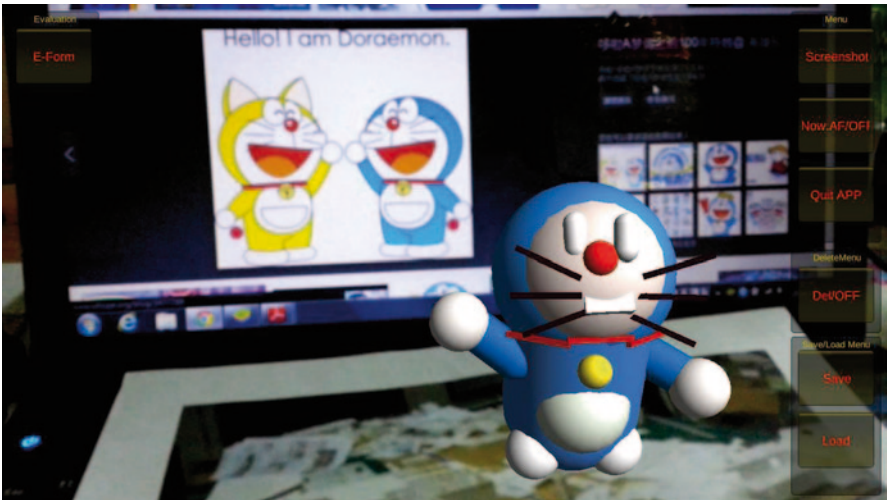
Fig. 26 A 3D model built by moving the primitive shapes via AR markers. (Tang 2015)
