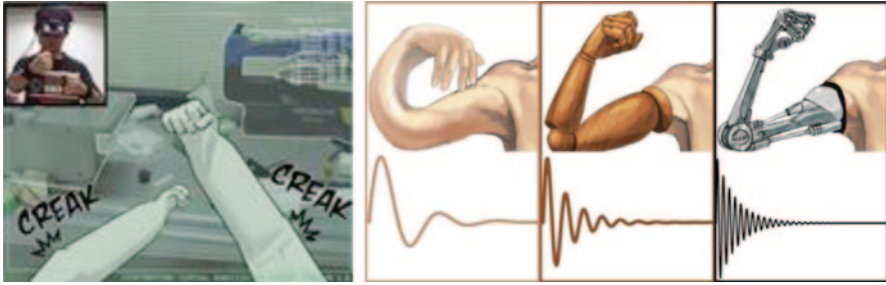
Fig. 34 The Jointonation system renders an impact vibration to the multiple joints, when the player's motion stops. (Kurihara et al. 2013)
