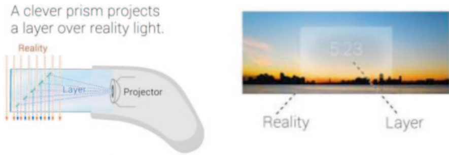
Fig. 21 The curved mirror optics technique is adopted in Google GLASS ( left ). The user's view is illustrated ( right ) (Missfeldt 2013)
