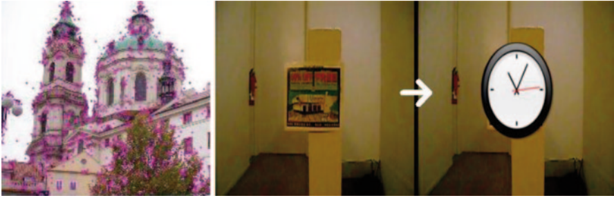
Fig. 9 An example AR application by SIFT algorithm (Matas et al. 2002). The key points located by SIFT ( left ). The virtual object displayed on the identified real object ( right )
