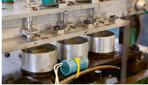
Fig. B7 Close up of the wear testing machine, the vertical rods have plastic tips that moved against the metal circular discs
