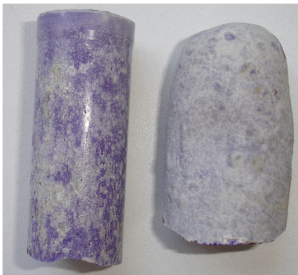
Fig. 14.1 Cement after bleaching. On the left : Injection moulded cement with a smooth surface finish showing patchy areas of bleaching. On the right : cement with an irregular rough finish with more extensive bleaching
