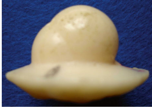
Fig. 32.1 Acrylic cast used to measure the real penetration of the cup
