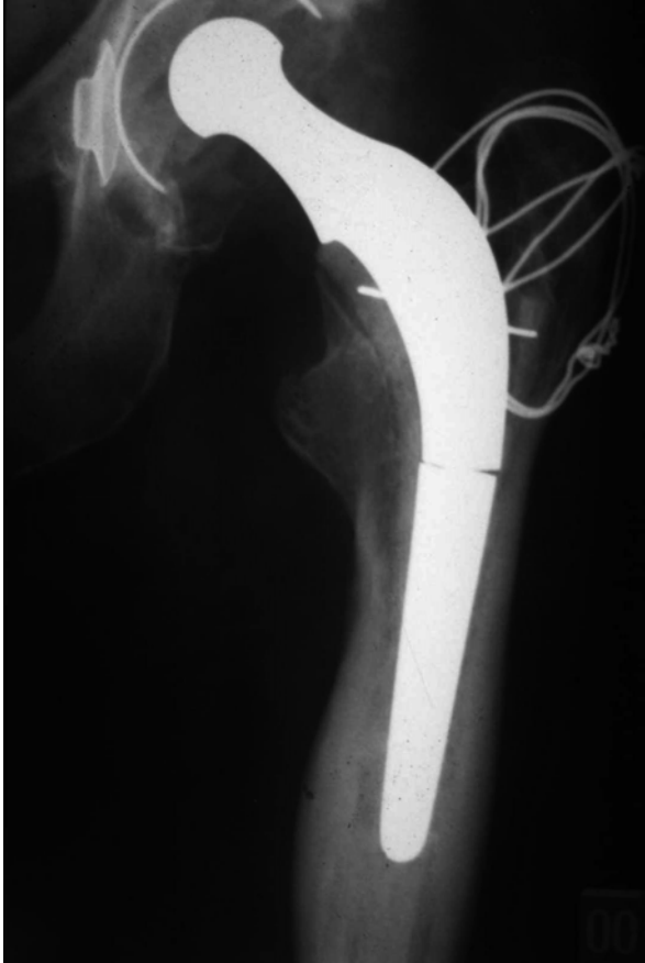
Fig. 24.2 Radiograph showing proximal strain shielding and distal strain concentration. Proximally this presents as loss of cortical definition and stem fracture
