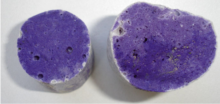
Fig. 14.2 Cement after bleaching. On the left : Injection moulded cement. On the right : cement with an irregular rough finish. Deeper layers are not bleached in both specimens. This demonstrates the limitations of cement spacers for antibiotic release
