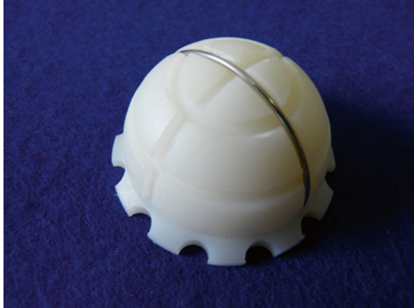
Fig. 27.14 Wire marker to measure wear the UHMWPE cup – the original version. (see radiograph Fig. 27.4)
