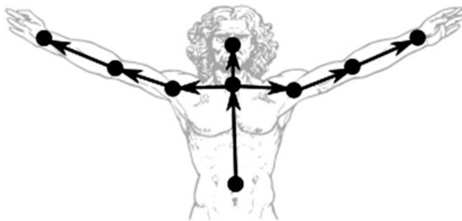
Fig. 6.4 The vectors of the upper body created for exercise evaluation are represented as arrows . The dots represent the body joints detected by a skeleton detection
