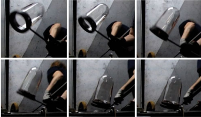
Fig. 5 Change in image characteristics of a glass object in the visual spectrum. The series of 6 consecutive images is taken during 1 s, approximately 11 s after the last series from the image in Fig. 4. The object formed has a temperature of approximately 700 °C
