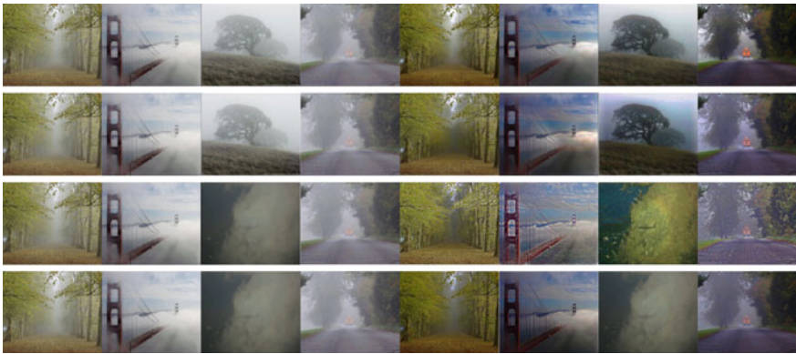
Fig. 3 Haze removal results of fog based on physical model, left the original images, right the haze-free images. From top to bottom dark channel prior, guided filter, NBPC, average filter
