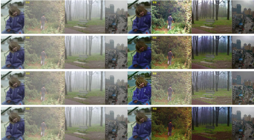
Fig. 1 Haze removal results of mist based on physical model, left the original images, right the haze-free images. From top to bottom dark channel prior, guided filter, NBPC, average filter
