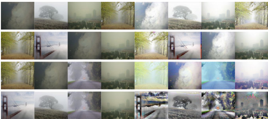
Fig. 4 Haze removal results of fog based on image enhancement, left the original images, right the haze-free images. From top to bottom FMR, RM99, MSRRCR, CLAHE
