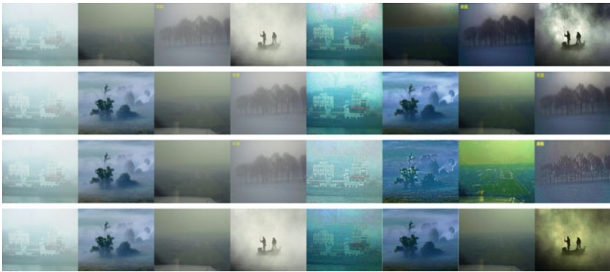
Fig. 5 Haze removal results of dense fog based on physical model, left the original images, right the haze-free images. From top to bottom dark channel prior, guided filter, NBPC, average filter
