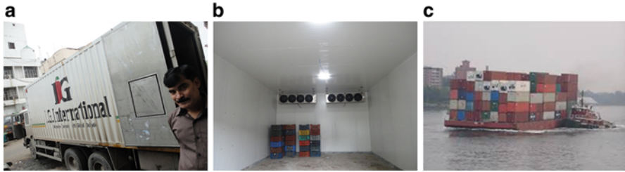
Fig 2.4 (a) Reefer container; (b) inside view of a reefer container; (c) ship loaded
