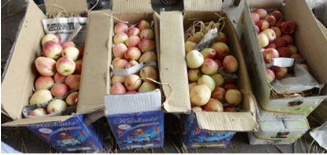
Fig. 3.6 Poor-quality CFB boxes
