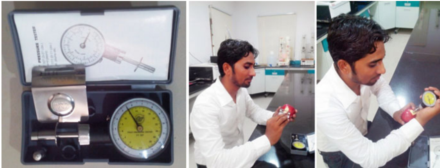
Fig. 13.4 Penetrometer box ( left ) with two plungers and peeling knife ( middle ) and testing ( right ). Note ring marks on the plunger ( middle )
