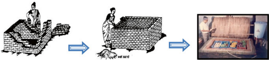
Fig. 9.1 Construction and operation of ZECC
